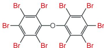
Decabromodiphenylether (Deca-BDE) is the only commercial product currently in use from the PBDE family. It has 10 bromine atoms attached to the diphenylether molecule, a high molecular weight and high thermal stability. Its major applications are in styrenic polymers, polyolefins polyesters, nylons and textiles. In May 2004, the Euro-
