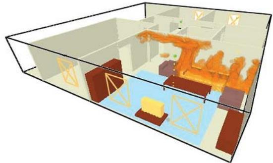
In these tests, the fires developed very rapidly after igniting either a TV or a bed mattress with a candle.
