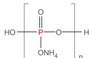
grades are primarily used in intumescent coatings. They are also used in rigid and flexible polyurethane foams and polyolefins (injection moulded), in formulations for unsaturated polyesters, phenolics, epoxies and coatings for textiles.
