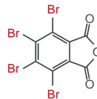
is often used as a reactive flame retardant in unsaturated polyesters used to manufacture circuit boards and cellular phones. It also serves as a raw material for the manufacture of other flame retardants.
