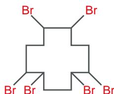
is a cycloaliphatic BFR. It is commonly used in foamed polystyrene for insulation of buildings where it is only necessary at very low loadings. For compact polystyrene (high impact) higher loadings are necessary. Another application is in textiles.
